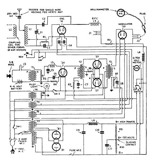
fig. 6. This modulated oscillator provided a 15 watt carrier. If properly built, the stability was passable and audio quality was quite good, considering a telephone microphone was used. The whole rig was breadboard construction on three shelves. Hams who could not afford a 10 transmitting tube, dropped the voltage and used a 245 or a 226, depending upon the state of their pocketbook.
